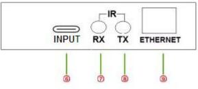
(1): **RS232**: RS232 port 2: LED HD-BaseT works well ,LED is blue ③: HD-BaseT HD-BaseT input (4): Power Power LED indicator (5): DC 5V 5V/2A power in 6: Input HDMI input (7): IR-RX **IR Receiver output** (8): IR-TX IR transmitter input (9): Ethernet Ethernet port
